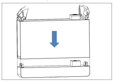
3. Lock screws into screw holes on both sides of the battery extension module, to ensure extension module is securely installed on the base; fasten wall anchor on the battery extension module, and then fasten it on the wall. Similarly, install other battery extension modules in turn and fasten them.
