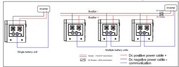
1a. For CPS SCE3.6/4.6/5/6KTL-60/120-EU inverter: If inverter connects to single battery unit or the first one of multiple networking battery units, connect the COM cable for SCE inverter to COM port of inverter and INV port of battery unit according to cable stickers, for the remaing networking battery units, choose standard Ethernet cable with the same connectors;
