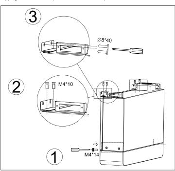
4. Fasten power control module onto the battery extension module. Then insert Dust caps into all the screw holes on the both sides.
