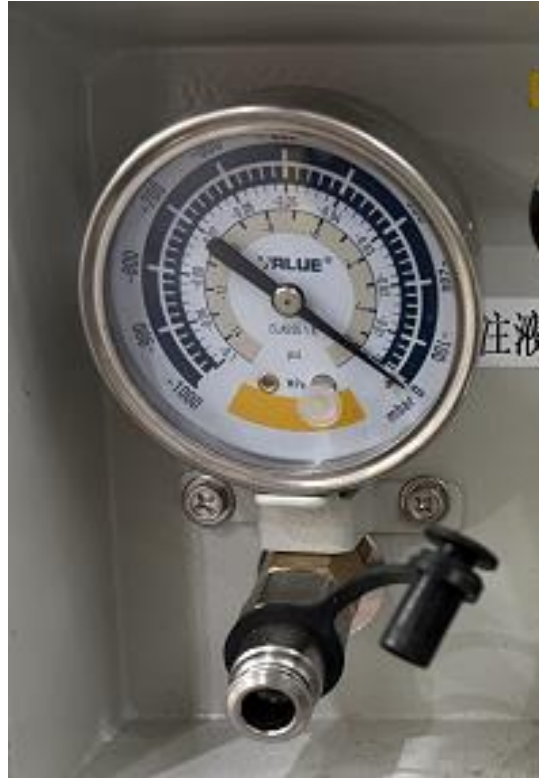
Fig. 9-16 Return water pressure
