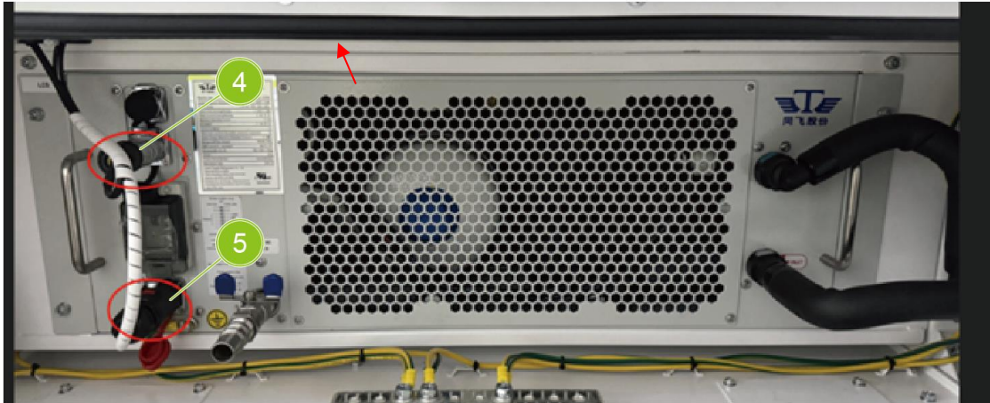
Fig. 9-8 Disconnect the communication cables
