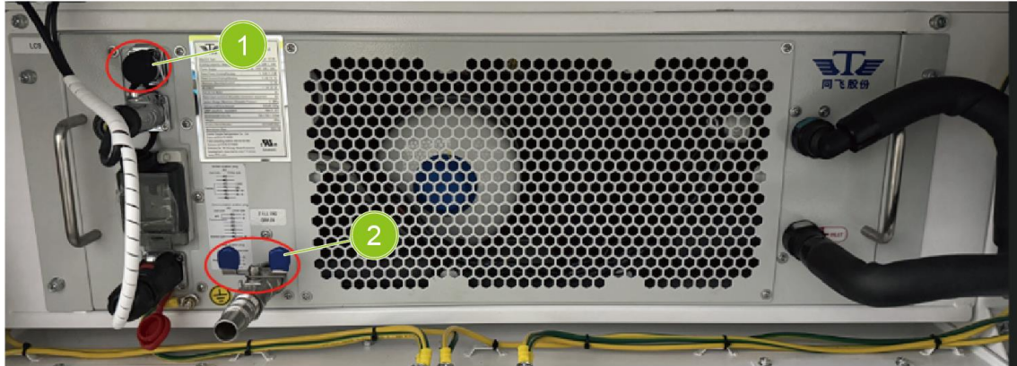
Fig. 9-12 Connect the quick plug and close the drain valve
