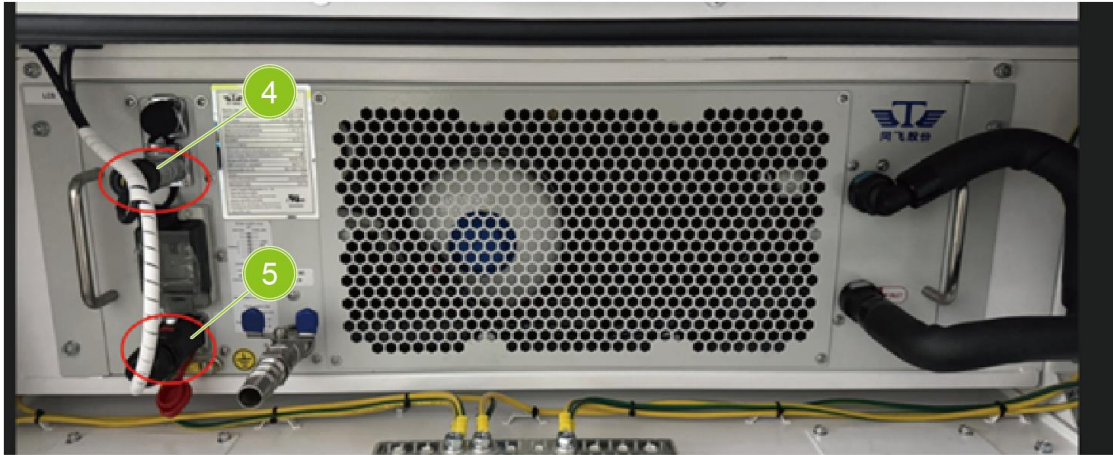
Fig. 9-12 Disconnect the communication cables
