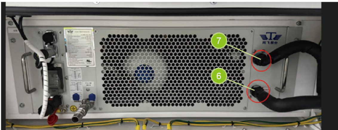
Fig. 9-13 Remove the coolant inlet and outlet pipes
